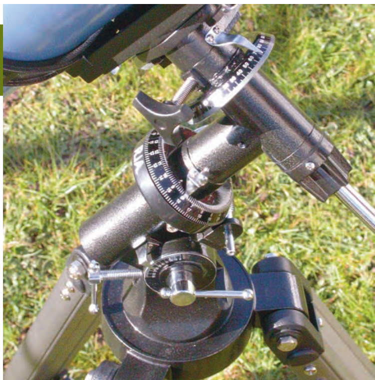
Left: The EQ2 German equatorial mount sports setting circles and slow motion controls on both axes. A relatively lightweight mount, it handles the Explorer-130PM with ease. Vibration damping time is in the region of three seconds.
